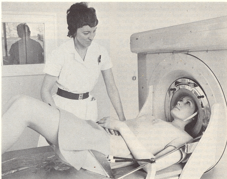
Fig. 2. Mk 1 brain scanner installed at Atkinson Morley Hospital, September 1971 definition 80 \times 80 later on 160 \times 160 . (Photo courtesy of EMI Ltd.)
